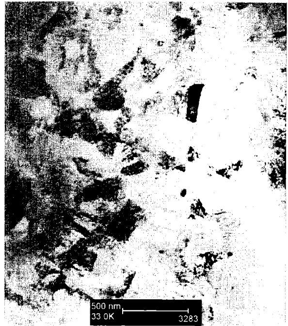
b) The SiC coating contains small, equiaxed grains, but no silver
